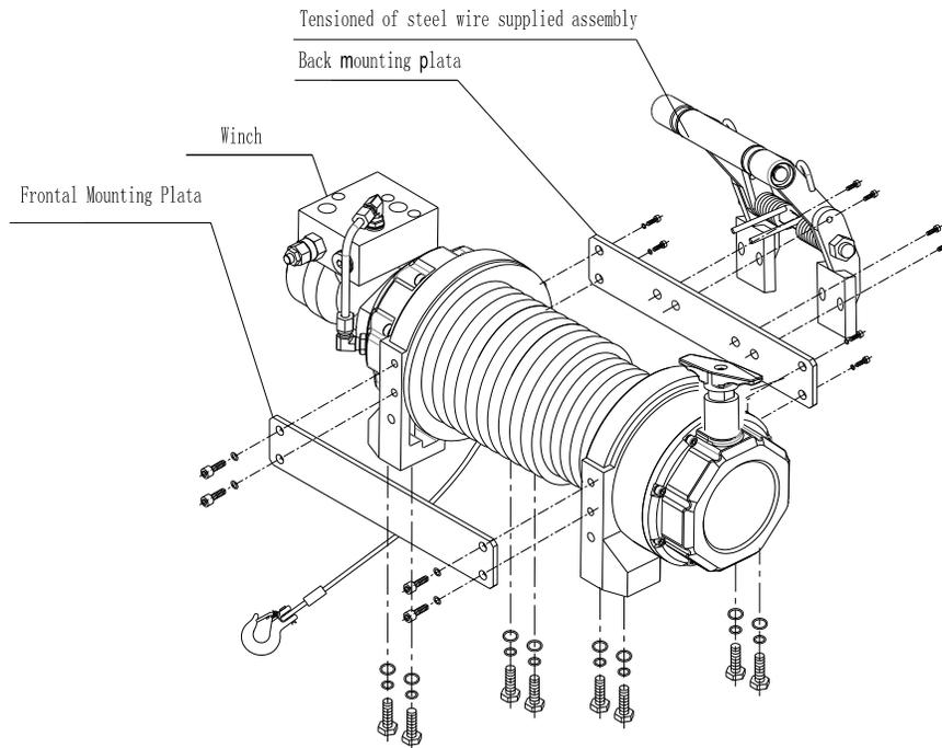
**Below is installation illustration with roller fairlead of winch:**
